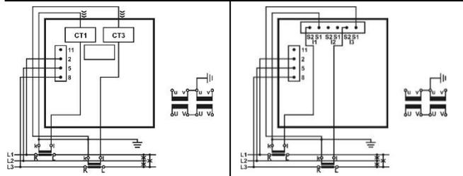
**Three-phase three-wire connection with unbalanced load 3u (2W3)**
