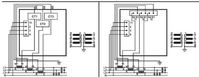
**Three-phase four wire connection with unbalanced load 4u (3W4)**
