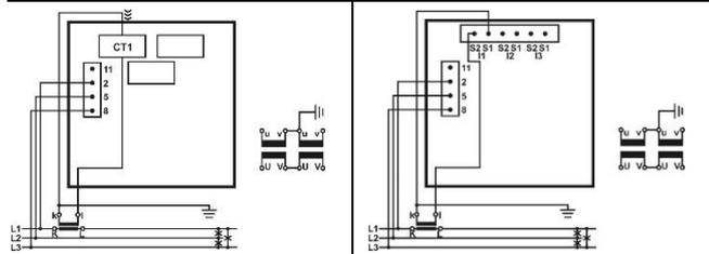
**Three-phase three-wire connection with balanced load 3b (1W3)**
