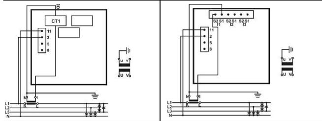
**Three-phase four wire connection with balanced load 4b (1W4)**
